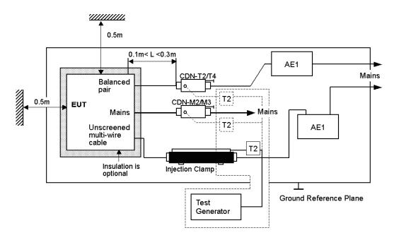
NOTE: The EUT clearance from any metallic obstacles shall be at least 0.5m. All non-excited input ports of the CDNs shall be terminated by  $50\,\Omega$  loads.
