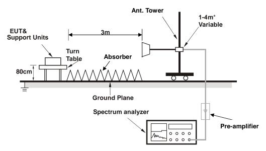
\*: depends on the EUT height and the antenna 3dB beamwidth both, refer to section 7.3 of CISPR 16-2-3.
